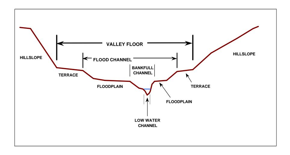
FIGURE 2.8: IDEALIZED VALLEY FLOOR CROSS-SECTION SHOWING TYPICAL GEOMORPHOLOGIC FEATURES.
