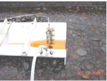
Figure 5. Flow monitoring station photographs. The left shows the flume and flow monitor and the right shows a close-up of the flume during a storm event.
