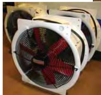
reached 115°F. This temperature is adequate for killing bed bugs but not high enough to damage belongings. This treatment will take 4 hours or longer.
