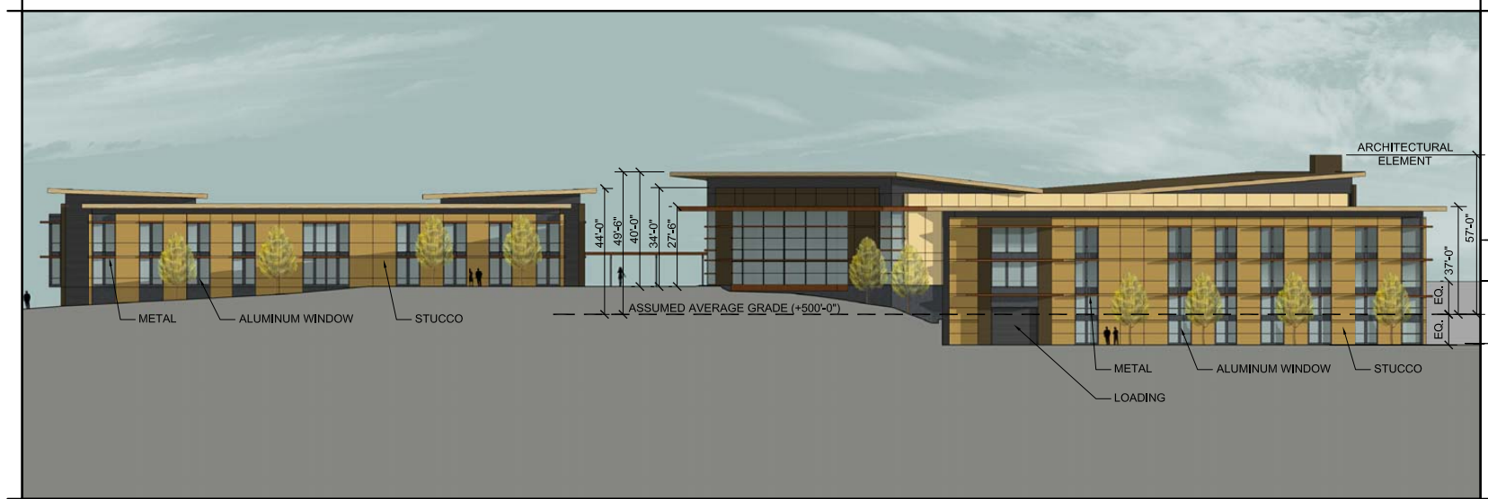
CHURCH AND ADMINISTRATION BUILDINGS: SOUTH ELEVATION
